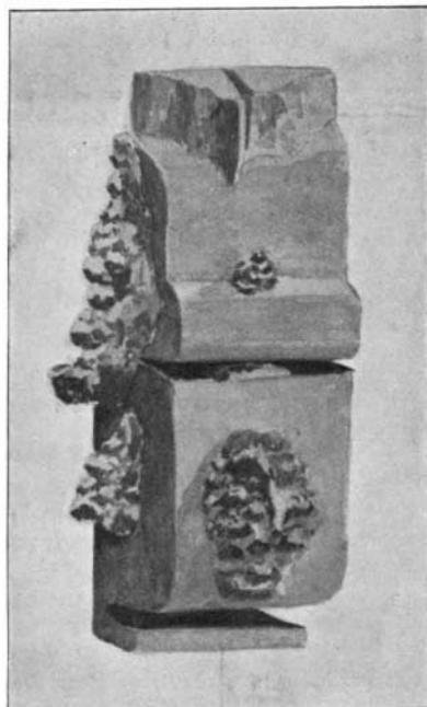
LUG FROM DEFECTIVE ELECTRIC WELD.
