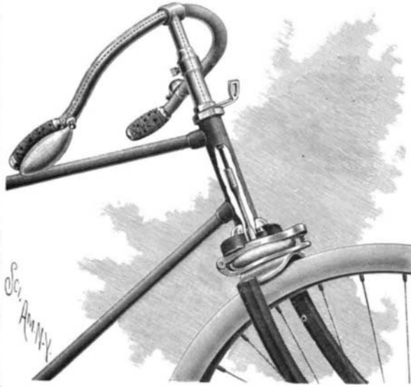
WALLACE'S PNEUMATIC BICYCLE BRAKE.
