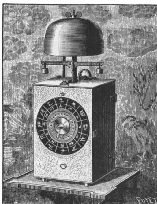
Fig. 2.—JAPANESE CLOCK WITH WEIGHTED BALANCE.
