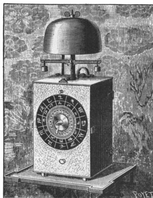
Fig. 2.—JAPANESE CLOCK WITH WEIGHTED BALANCE.
