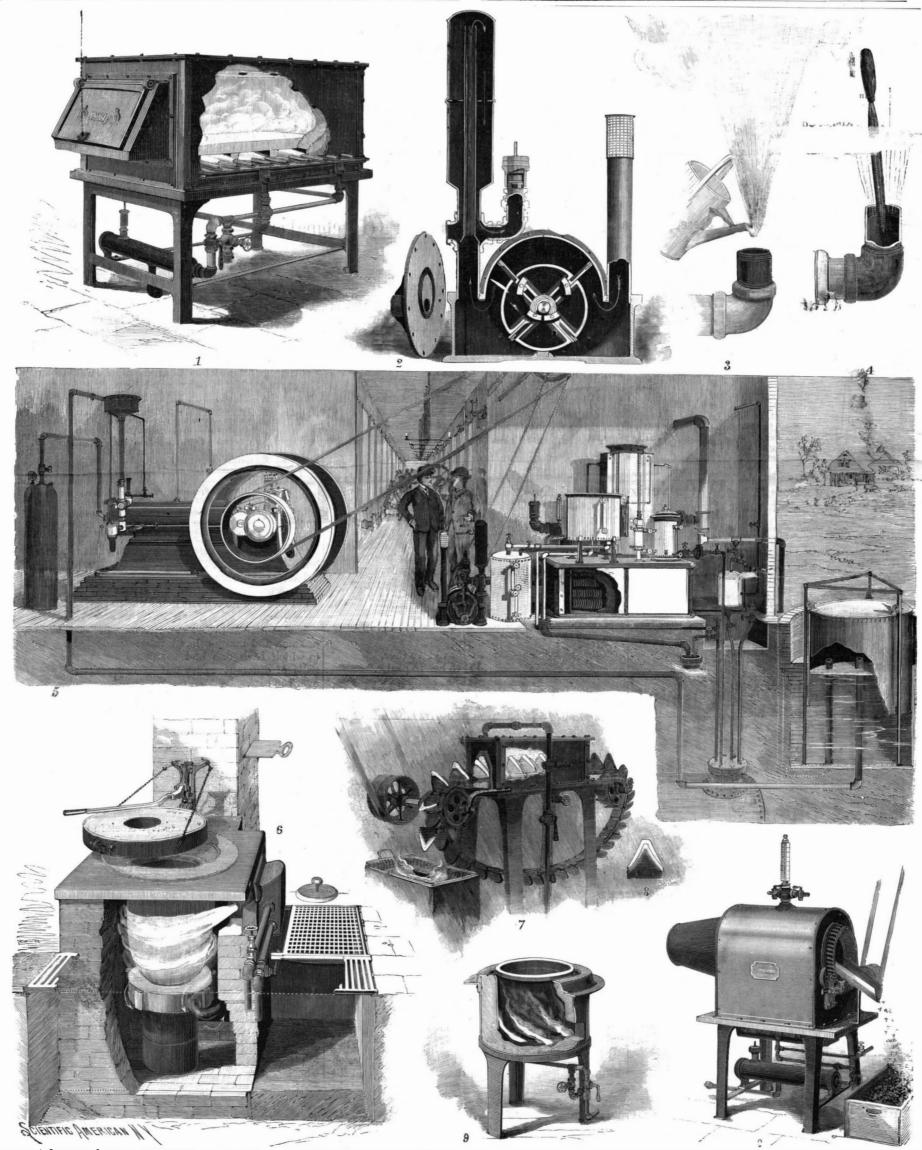
1. Large oven furnace. 2. Rotary blower. 3 and 4. Experiments with the blast. 5. The gas-producing plant 6. Large melting furnace. 7. Furnace for tempering mowing machine cutters. 8. Soft metal furnace.
