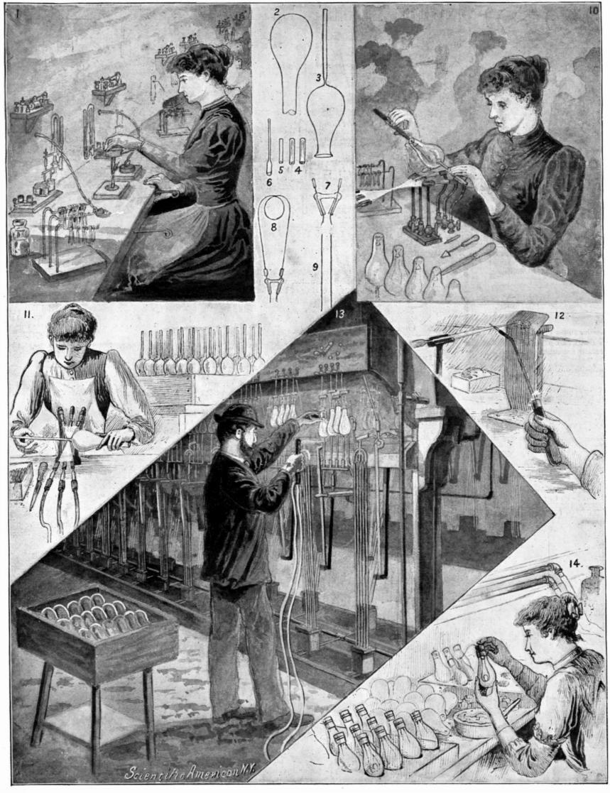
4. Flashing in. 2. Bulb. 3. Tubulated bulb. 4. Insulating tubes. 5. Bridge. 6. Platinum leading-in wires. 7. Mount. 8. Mount and filament complete. 9. Copper connecting wires. 10. Sealing and sinking. 11 Tubulating. 12. Insulating. 13. Exhausting. 14. Capping.
