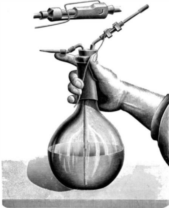
WASH BOTTLE IN USE, WITH VIEW OF VALVE.
