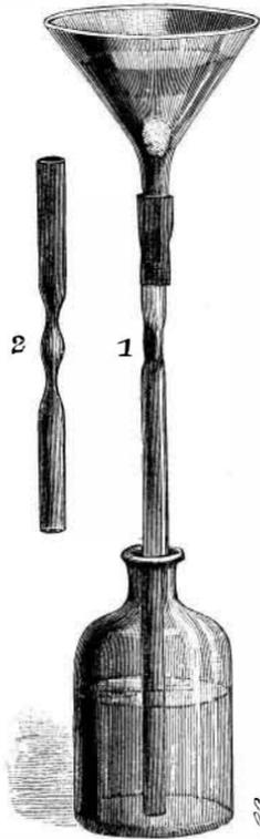
**RAPID FILTERING APPARATUS.**
