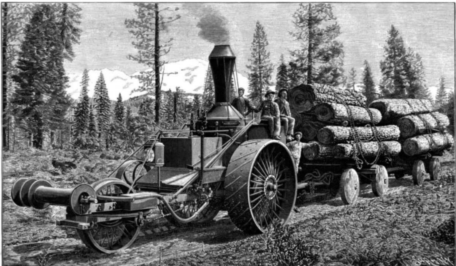
**TRACTION ENGINE USED FOR LOGGING PURPOSES IN CALIFORNIA.**
