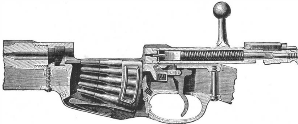
THE MANNLICHER RIFLE, SHOWING THE CHARGE BEING INTRODUCED AND THE BREECH OPEN.
