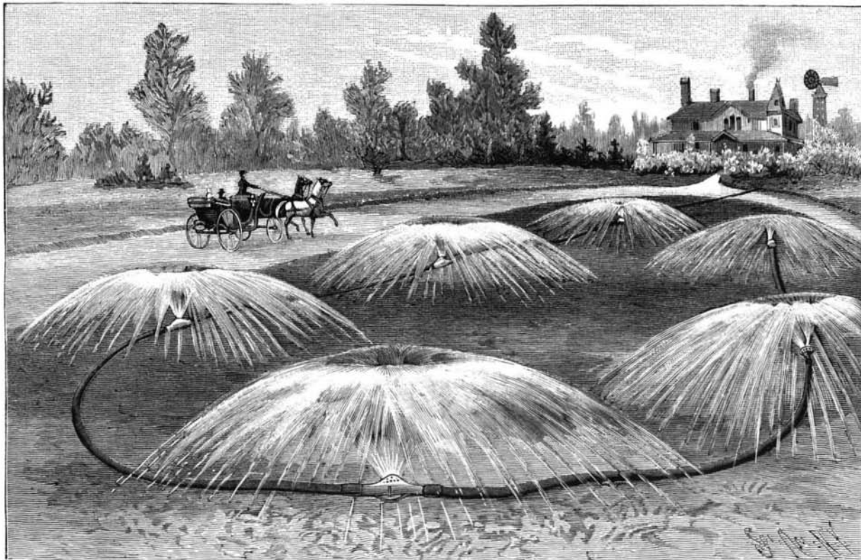
Fig. 1.—FOUNTAIN PIPES FOR LAWN IRRIGATION.
