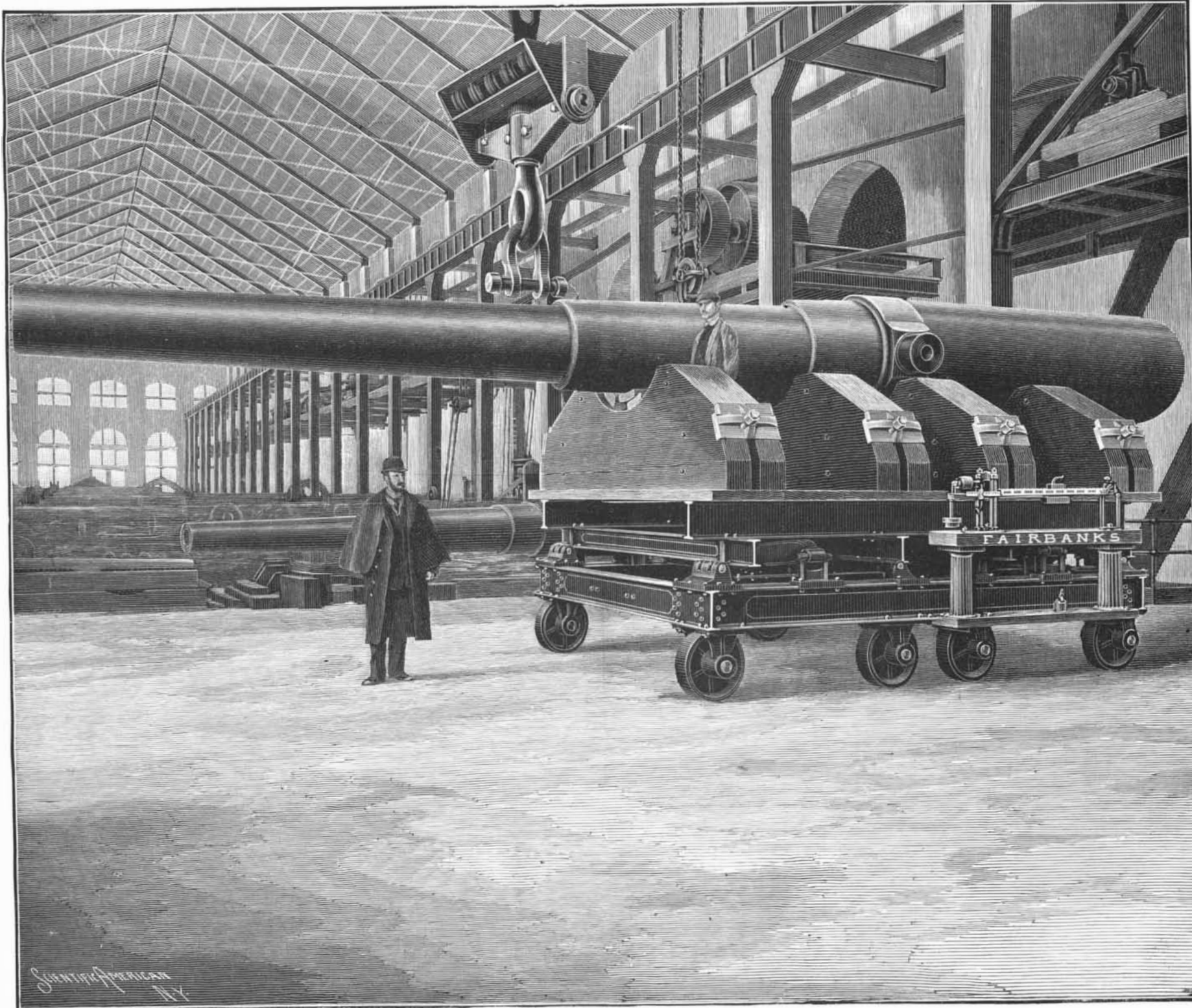
THE ONE HUNDRED AND FIFTY TON GUN SCALE OF THE WATERVLJET ARSENAL.
