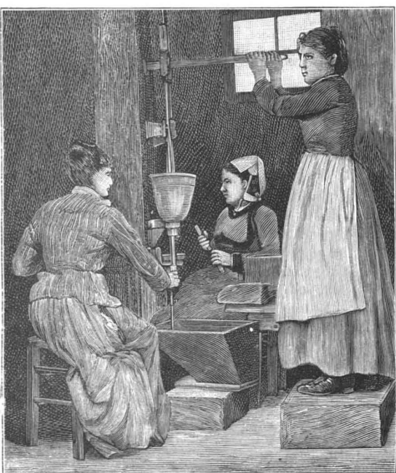
Fig. 5.—FILLING THE CARTRIDGES BY MACHINE.
