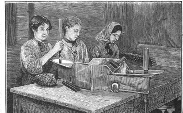
Fig. 4.—FILLING THE CARTRIDGES BY HAND.
