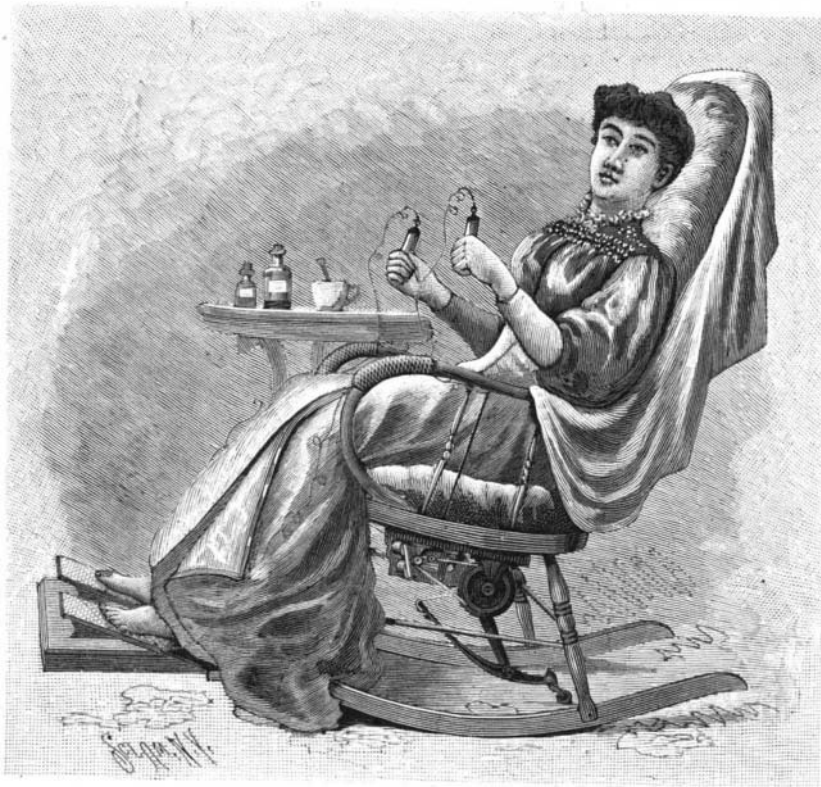
HARTELIUS' ELECTRICAL ATTACHMENT FOR ROCKING CHAIRS.
