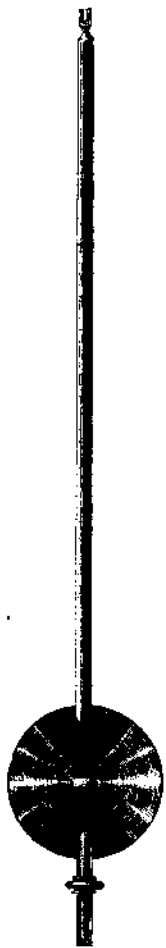
Riefler's Mercurial Compensation Pendulum.
