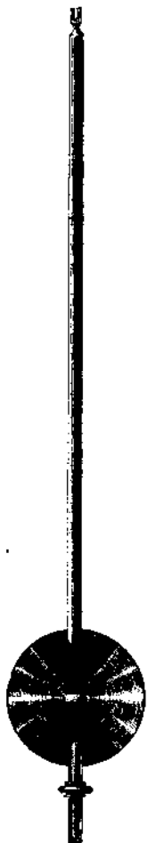
Riefler's Mercurial Compensation Pendulum.
