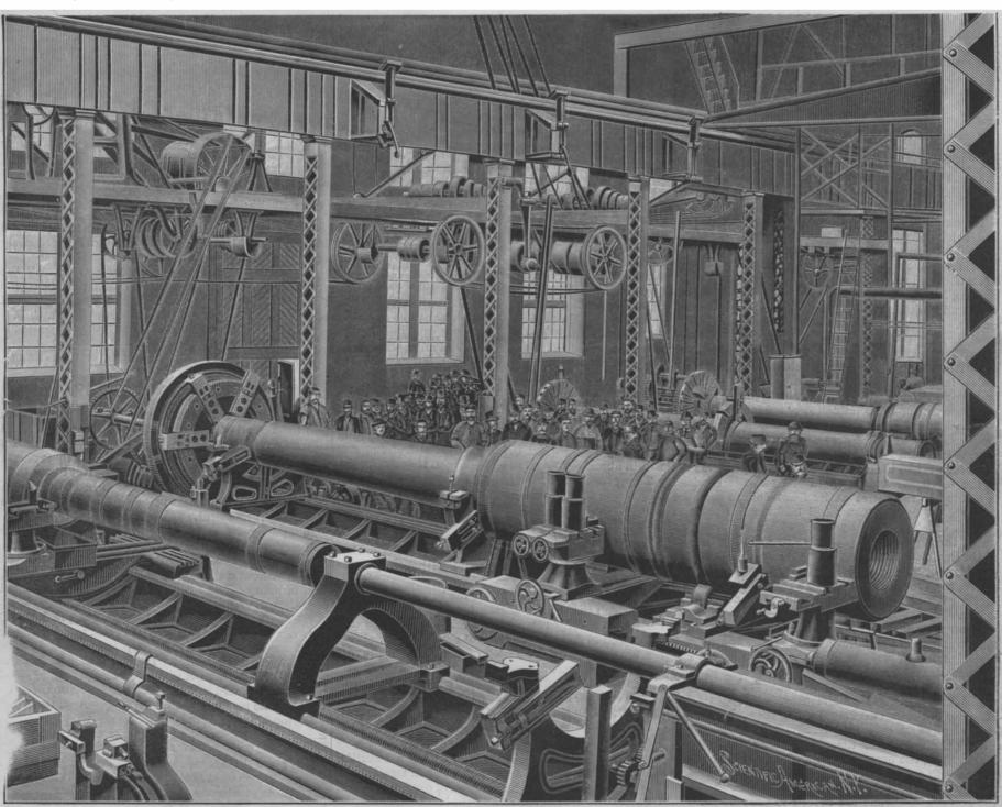
BORING, TURNING, AND CHAMBERING HEAVY GUNS AT THE WASHINGTON GUN FACTORY.
