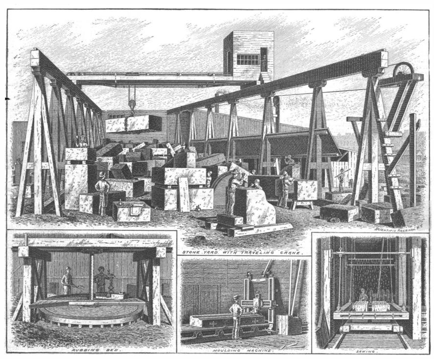
ILLUSTRATIONS OF STONE CUTTING, SAWING, AND POLISHING.
