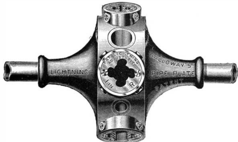
GALLOWAY'S "LIGHTNING" DIE STOCK FOR PIPE.
