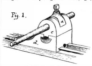
shows the contrivance employed. The block, c, was of cast iron, and the holder, a, of best refined iron, the lower end being gibbed into the rest, d, and a hole through the center sufficiently large to allow the boring bar to pass without touching, so that when the set screw was tightened, the whole was made fast to the lathe rest. d.
