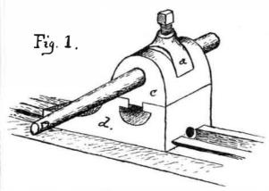
shows the contrivance employed. The block, c, was of cast iron, and the holder, a, of best refined iron, the lower end being gibbed into the rest, d, and a hole through the center sufficiently large to allow the boring bar to pass without touching, so that when the set screw was tightened, the whole was made fast to the lathe rest. d.
