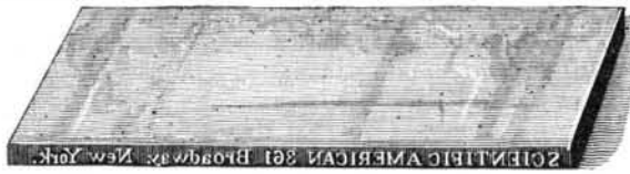
A LINOTYPE, OR TYPE BLOCK OF ONE LINE.
