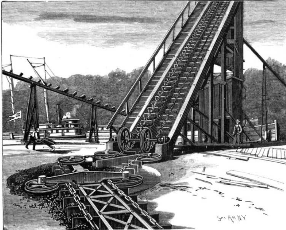
THE RELOADER SHOWING METHOD OF RAISING AND DELIVERING COAL INTO THE BARGE.
