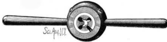
Fig. 2.—SCREW PLATE WITH BRION'S DIE.
