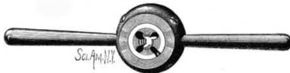
Fig. 2.—SCREW PLATE WITH BRION'S DIE.
