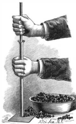
FIG. 2.—MOULDING CARBON RODS.
