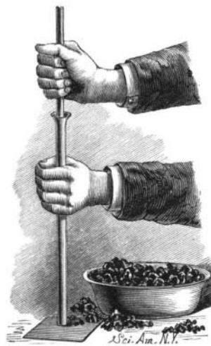
Fig. 2.—MOULDING CARBON RODS.
