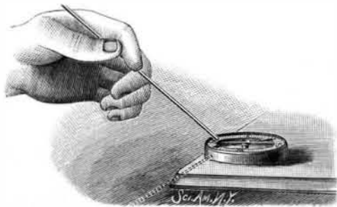
Fig. 1.—MAGNETISM BY INDUCTION FROM THE EARTH.
