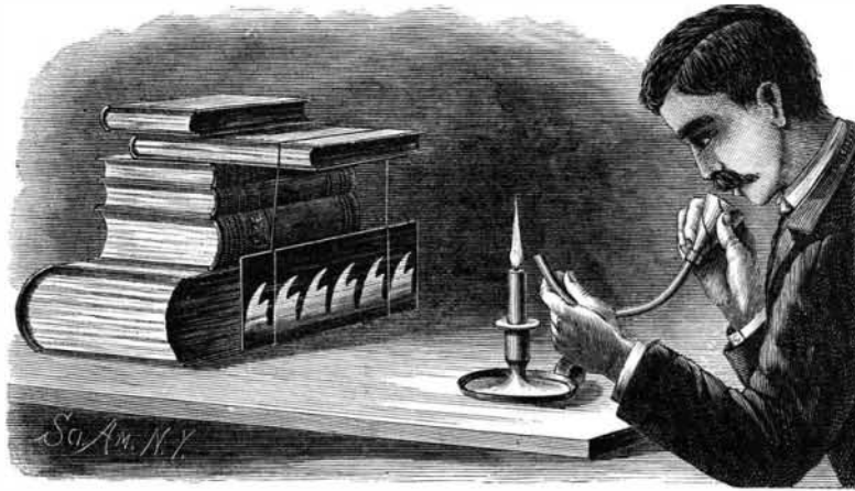
Fig. 1.—SIMPLE METHOD OF PRODUCING AND VIEWING VIBRATING FLAMES.
