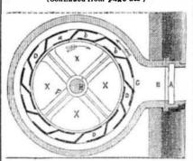
GWYNNE'S WATER WHEEL .- This engra ing, fig. 55, is a sectional elevation of a water wheel, recently patented in England, and termed "Gwynne's Patent Double Acting Balance Pressure Wheel." A swelling name truly.
