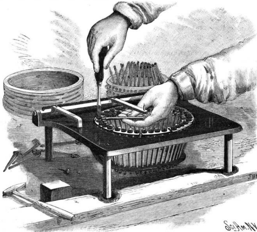
Fig. 10. - CENTERING THE TYPE ARMS.
