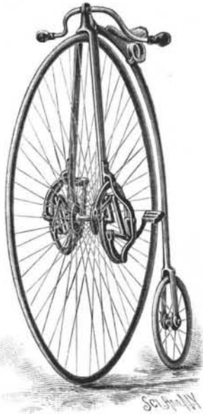
HANLEY'S CRANK APPLIED TO A BICYCLE.
