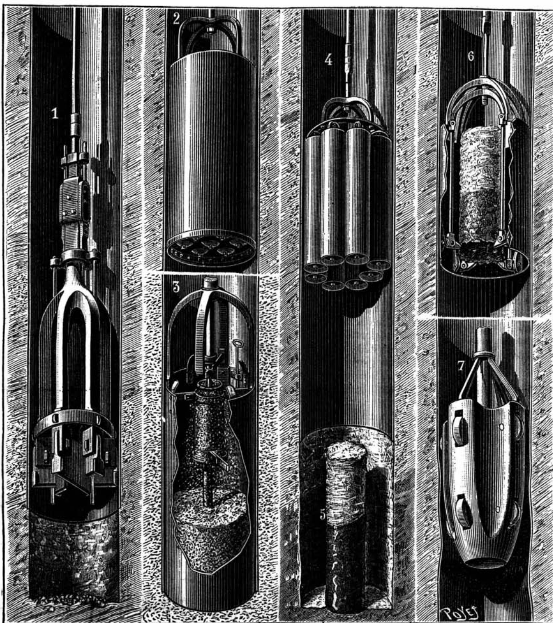
Fig. 2.—INSTRUMENTS USED FOR BORING THE ARTESIAN WELL IN THE PLACE HEBERT, PARIS.
