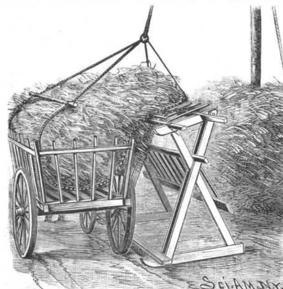
HOYT'S HAY UNLOADER AND STACKER.
