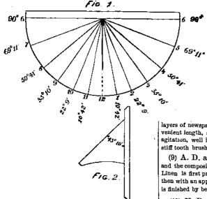
a plan and Fig. 2 a section through style. Such a dial keeps only mean time, and you will have to consult almanac as to when the sun is fast and slow. 2. The bestcement to mend rubber coats and boots. A. For mending rubber goods, use rubber cement, which can be obtained from the dealers in rubber goods. See SUPPLEMENT, No. 158, for numerous cements.
