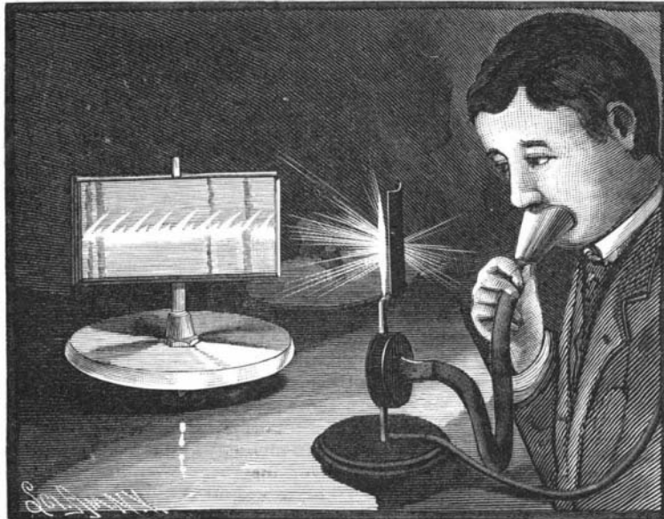
Fig. 1.—TOP WITH REVOLVING MIRRORS—KÖNIG'S MANOMETRIC FLAMES.
