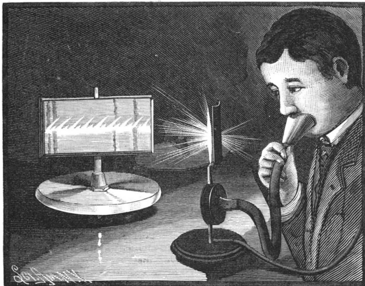
Fig. 1.—TOP WITH REVOLVING MIRRORS—KÖNIG'S MANOMETRIC FLAMES.
