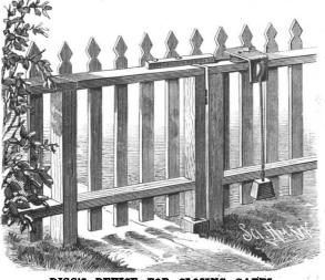
RIGG'S DEVICE FOR CLOSING GATES.
