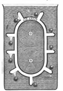
weight is attached to each bag. The bags are filled with air when the weight hangs down, and when it comes on top it presses the air out and through the hollow projection and tube into the next bag that comes in position. When placed over two wheels in water, the bags filled with air should be lighter and rise, while the other side with the air forced out should sink."
