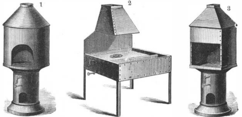
EHGOTT'S IMPROVEMENTS IN PORTABLE FORGES.
