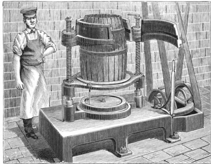
Fig. 2.—MACHINE FOR ASSEMBLING STAVES.
