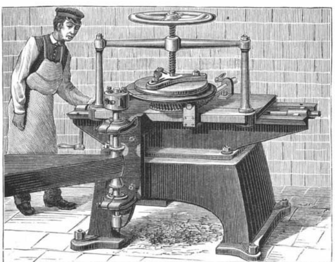
Fig. 4.—MACHINE FOR TURNING AND CHAMFERING BARREL HEADS.
