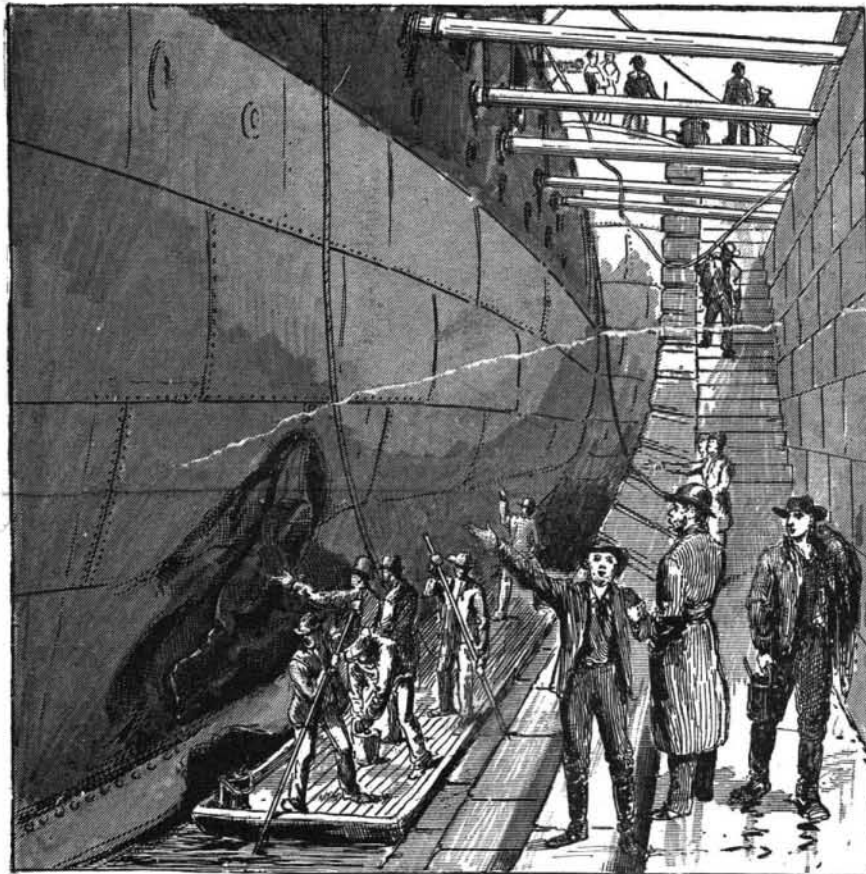
TORPEDO EXPERIMENTS AT PORTSMOUTH—DAMAGE DONE TO THE PORT SIDE OF H.M.S. RESISTANCE.
