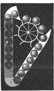
ing balls will force it out until it rolls off on to the proper place on the power wheel. Here the balls exert their weight, turn core and pushed into engagement with the teeth by a the wheel, and then drop back into starting channel to force the ones ahead of it through the mercury back into the water again.
