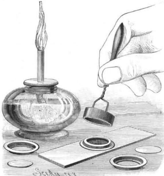
Fig. 1.—QUICK METHOD OF MOUNTING MICROSCOPIC OBJECTS.
