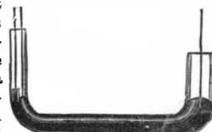
Fig. 5.—U TUBE OF UNDULATORY SEISMOGRAPH.
