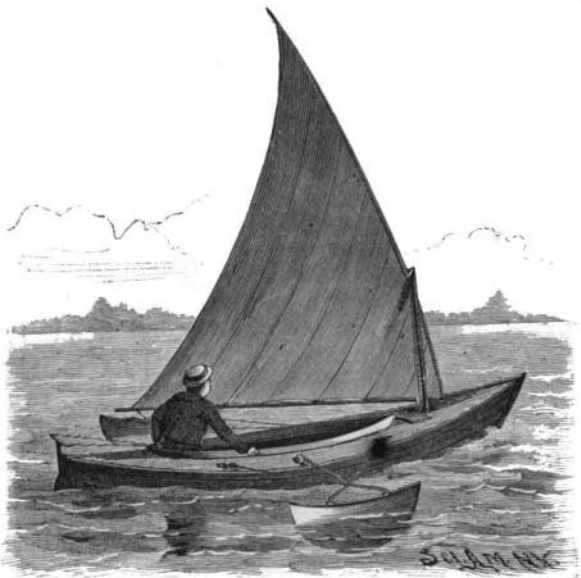
CLAPHAM'S LEE BOARD FOR SMALL VESSELS.
