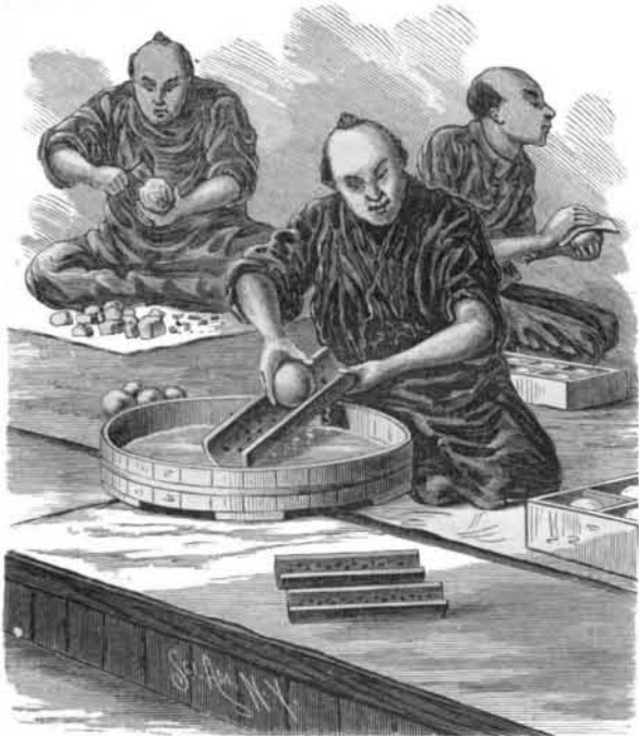
JAPANESE METHOD OF GRINDING CRYSTAL BALLS.
