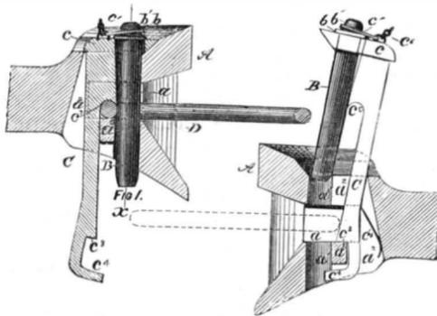
of C. M. Hoag, of Greenbush, an engineer on the Boston and Albany Railroad. At the trial it was the only one that made the "flying switch" automatically. In its normal condition the link is level, and works successfully on all cars. The recommendations of the commission, which are the most important made since its organization, are as follows:
