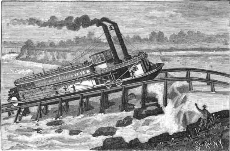
GRONDAHL'S APPARATUS FOR CARRYING VESSELS OVER OBSTRUCTIONS.
