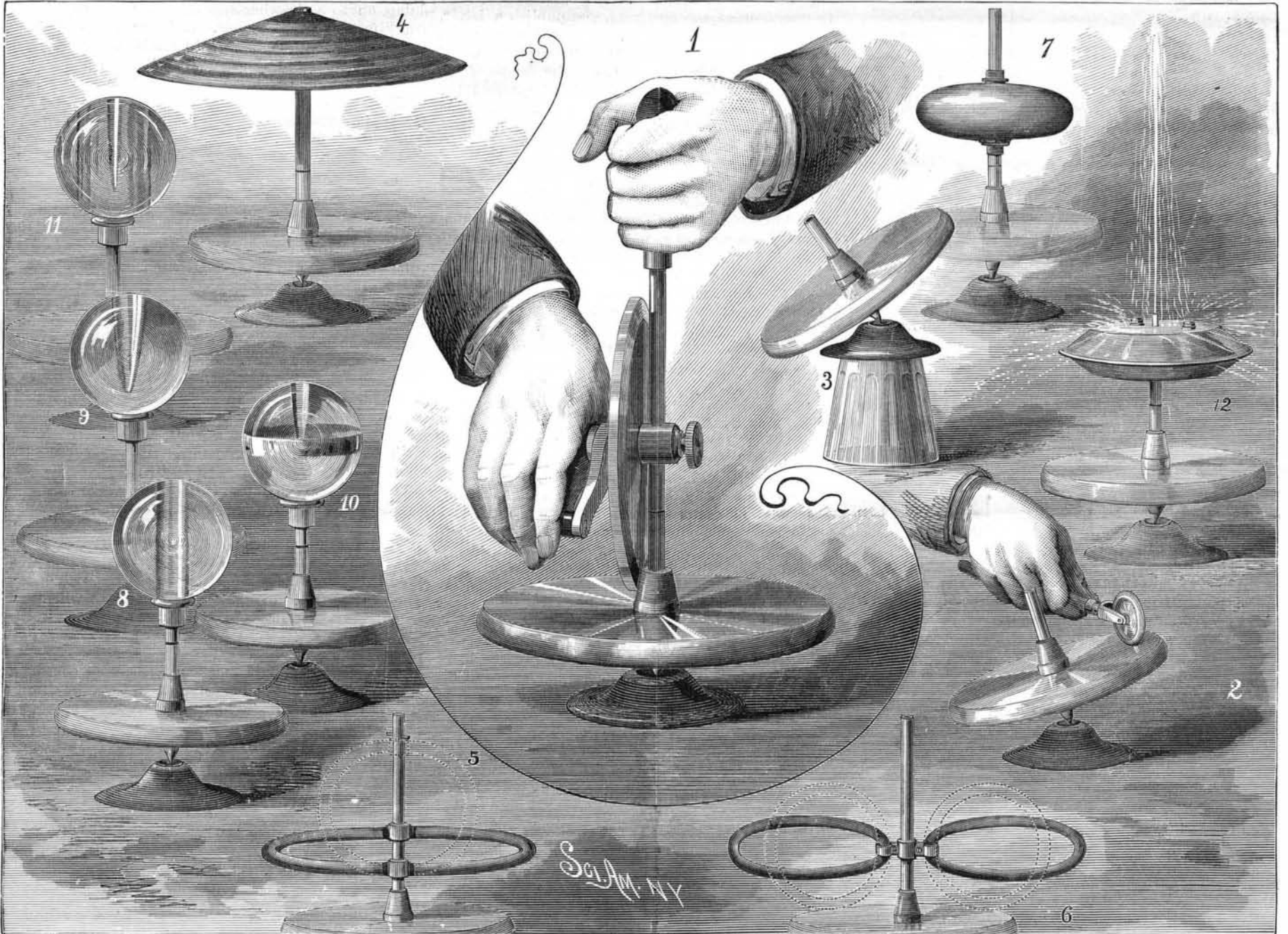
1. The Top. 2. Persistence in Maintaining Plane of Rotation. 3. Gyroscopic Action. 4, 5, 6. Examples of Centrifugal Action. 7. Formation of Oblate Spheroid. 8, 9, 10, 11. Examples of Centrifugal Action on Liquids. 12. Centrifugal Hero's Fountain.
