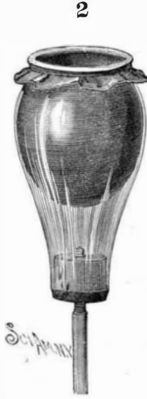
RUBBER FORCED INWARD BY AIR PRESSURE.
