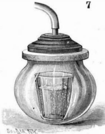
WATER BOILING IN VACUO.
