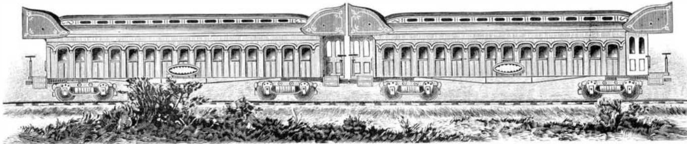
GILLHAM'S GUARD FOR RAILWAY CARS, TO KEEP SMOKE, DUST, ETC., FROM ENTERING THE DOORS.
